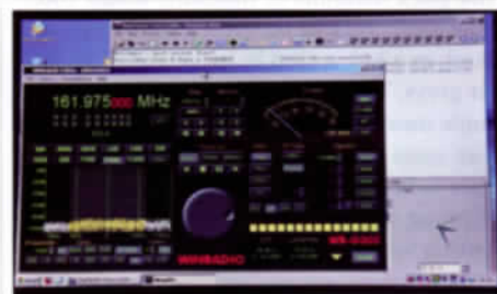
The Winradio receiver feeds AIS signals into a computer, which decodes and displays them.
